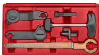
906G10 P.1-42 Engine timing tool for VAG
